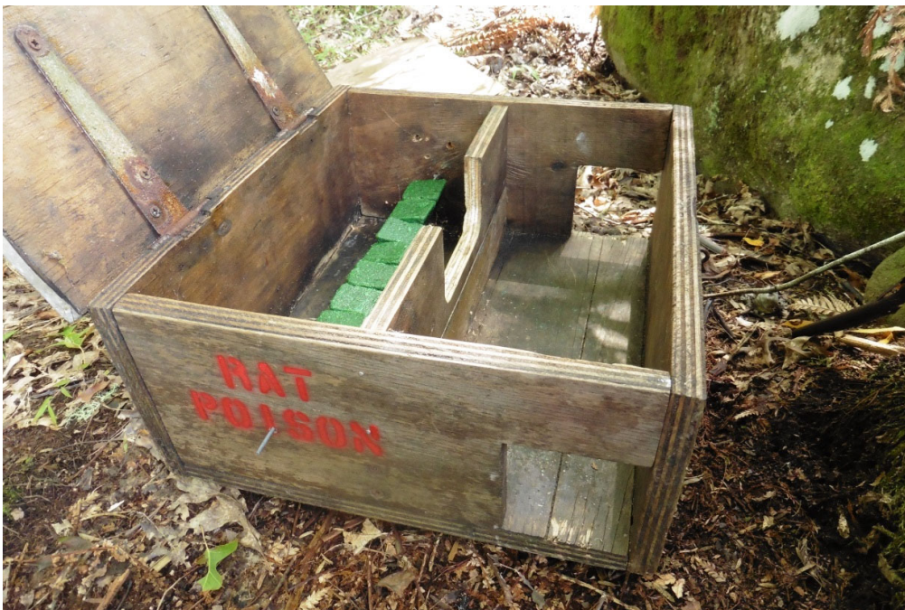
Photo 13. Rat poison box fitted with hasp and staple with a small rust-proof padlock. Note the possum proof centre baffle.
