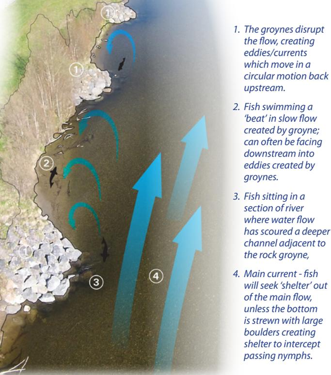
1. The groynes disrupt the flow, creating eddies/currents which move in a circular motion back upstream.
