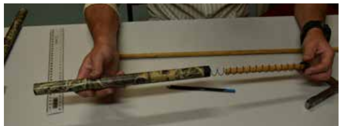
Figure 2. Place the dowel in the spring and return it to the magazine cylinder.
