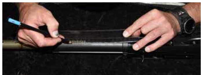
Figure 3. For the semi-auto measure 159mm from the breech end and place a mark.
