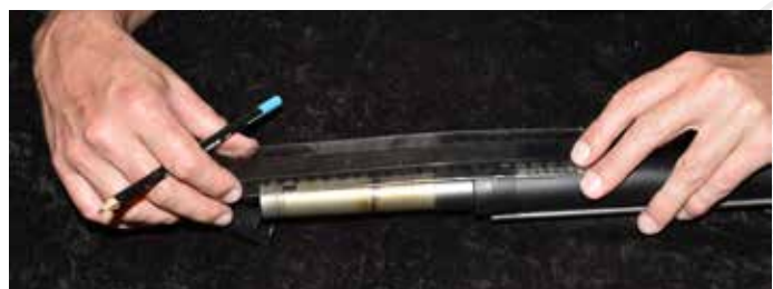
Figure 4. Measure from the mark to the end of the magazine or if there is an end stopper to this point. This is how long your dowel needs to be.
